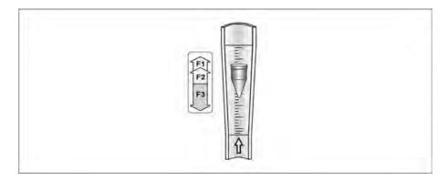
The height of the float is read on the scale of the measuring cone and indicates the flow rate.
